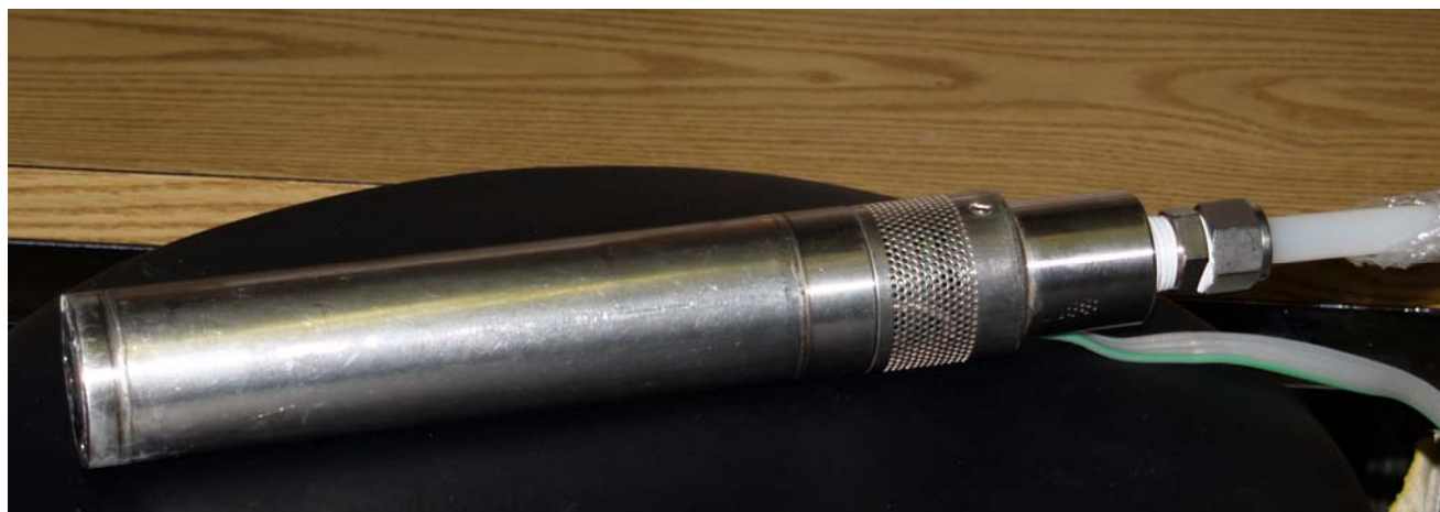
Figure 1 Grundfos/Rediflow 2 Submersible Pump and 13 mm Diameter Nylon Tubing Reel
