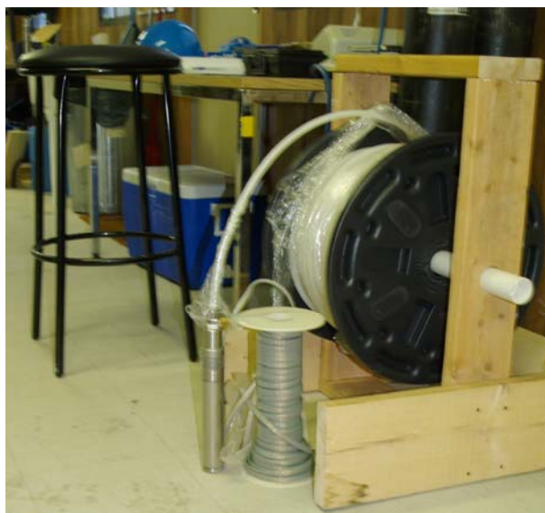
Figure 2 Close-up Photo of the Grundfos/Rediflow 2 Submersible Pump
